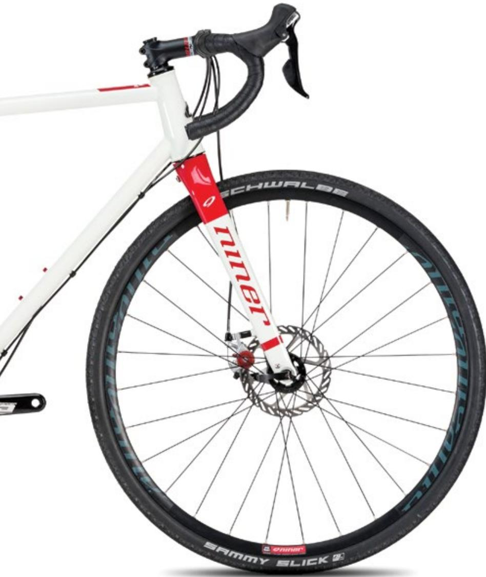
feature rack and fender mounts both front and rear. In fact with the updated fork that Niner unveiled in October 2015, the company offers the industry's few carbon fiber forks with mid-blade rack mounts (the Specialized Diverge is another).
