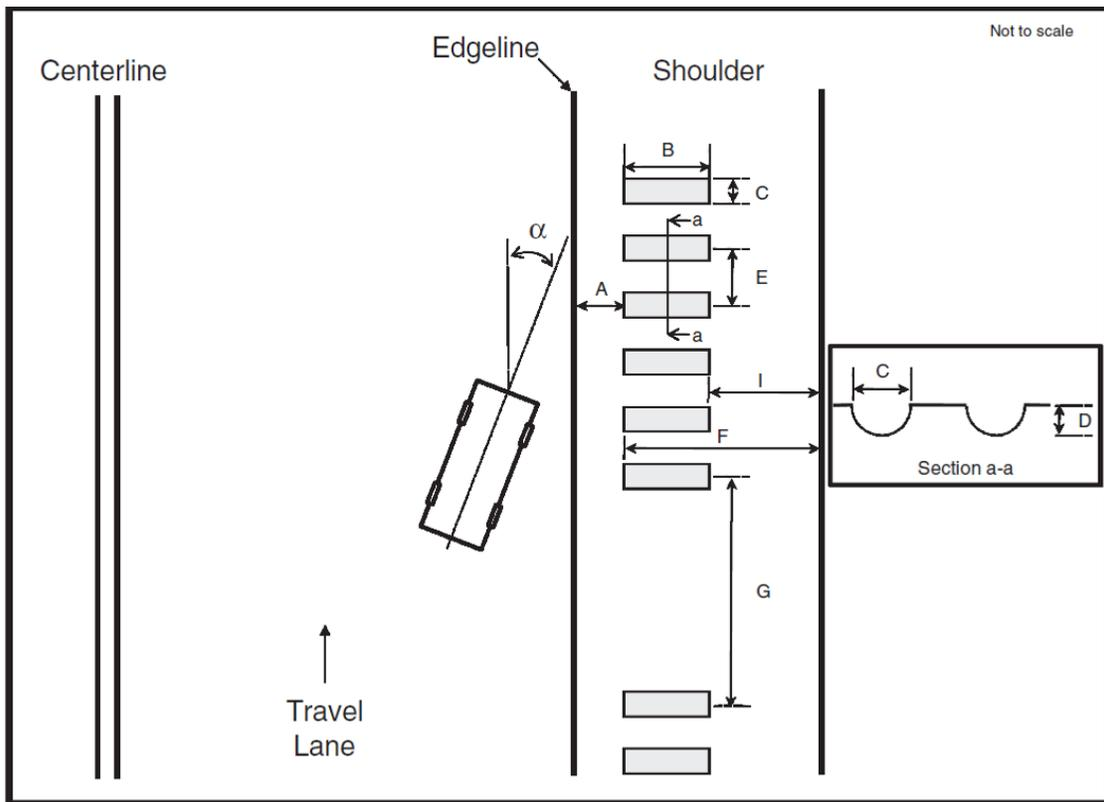
Figure 3. Design parameters associated with rumble strips. [Torbic 2009]
