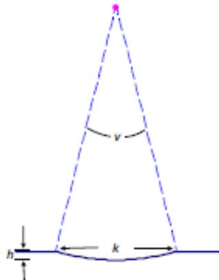
Figure 1. "Cylinder segment"; strip No. 1;  $h = 0.01$  m;  $k = 0.15$  m; strip width = 0.30 m;  $\lambda = 0.6$  m.
