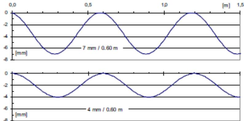
Figure 2. Sinusoidal; strip No. 2 (top) and No. 3 (bottom).
