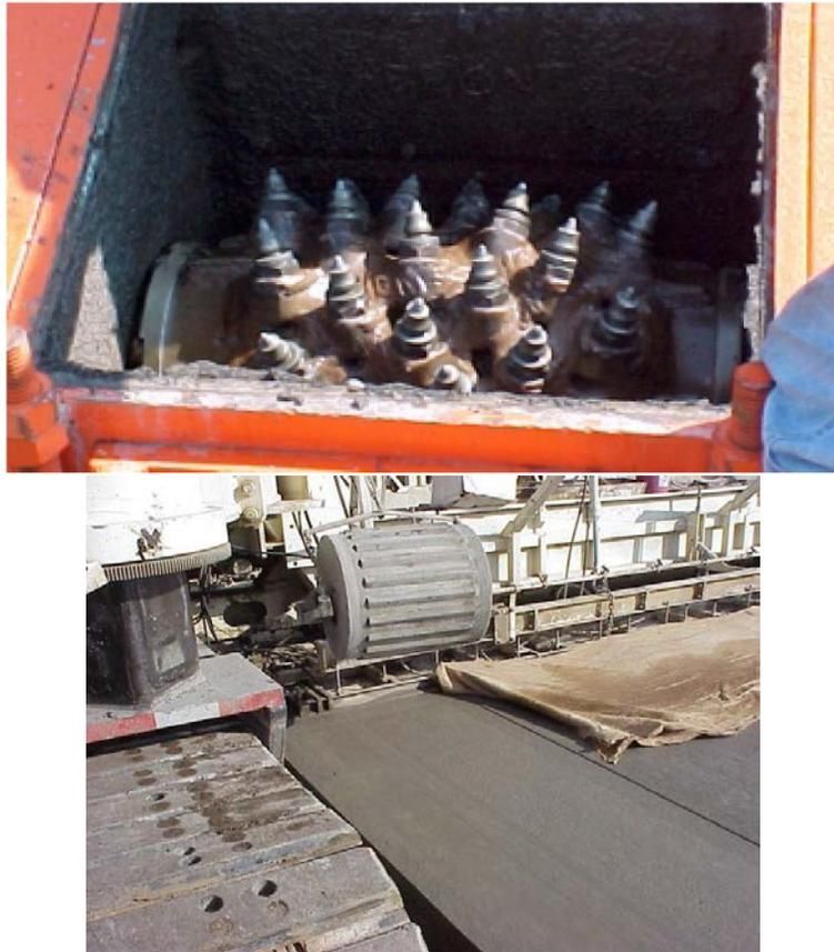
**Figure 2. Milling unit [Elefteriadou 2000] and formed-rumble-strip unit [Outcalt 2001-2].**
