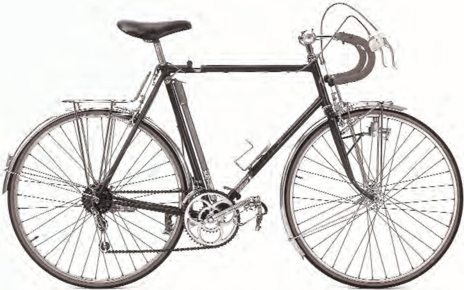
*This René Herse “coupler” bike was ordered by a member of the International Bicycle Touring Society in 1971. It features quick releases not only for the frame, but also the stem. Shift levers under the seat simplify the disassembly procedure, which takes less than 2 minutes.*
