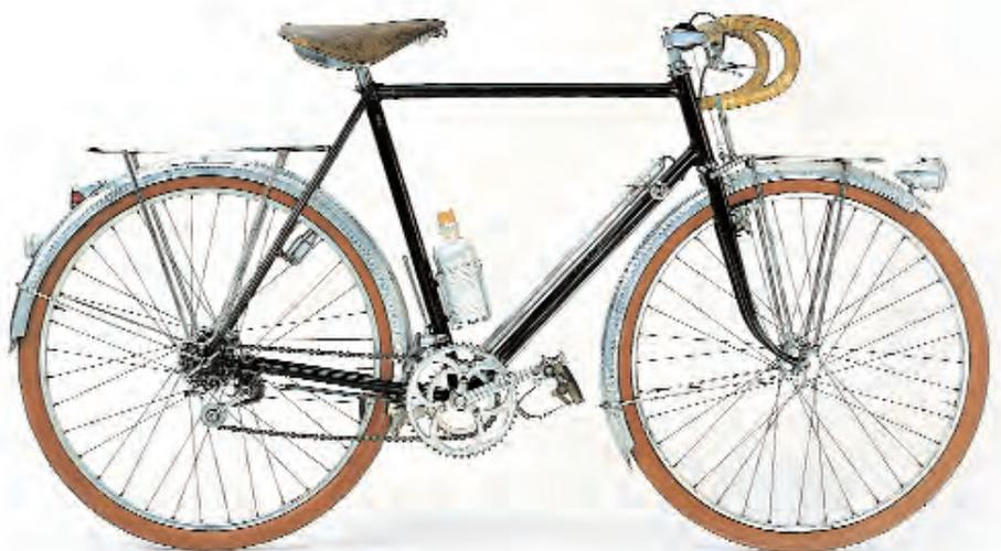
*“Camping” bikes like this 1948 René Herse were equipped with special geometries, sturdy racks made from steel tubing, as well as integrated lights and fenders. A rear drum brake allows descending unpaved mountain passes, which requires constant braking, without overheating the rim.*
