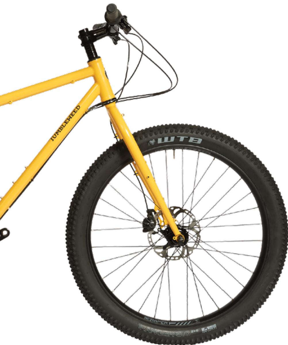
sand, a set of 26 x 4.0in. fat bike tires can be installed (but only with either a singlespeed drivetrain or an internal gear hub). If you want to maximize rollover in technical terrain, a set of 29+ wheels can do the job. And if you want to save a bit of weight, throw on a pair of 27.5+ wheels and tires.
