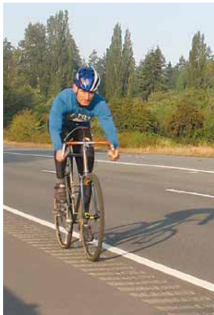
*Testing comfort on the rumble strips of a highway. The smooth surface next to the rumble strips provides a reference for comparison. Comparing power outputs for different setups quantified the power losses due to vibrations.*
