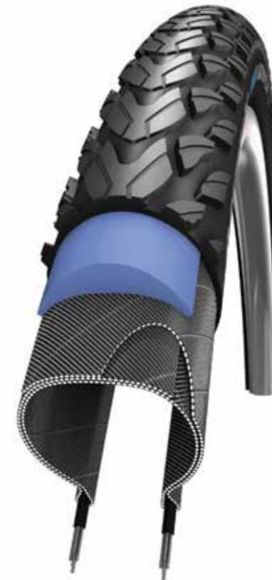
Figure 1: Puncture-resistant tires have tough belts and foam layers that decrease comfort and performance.
