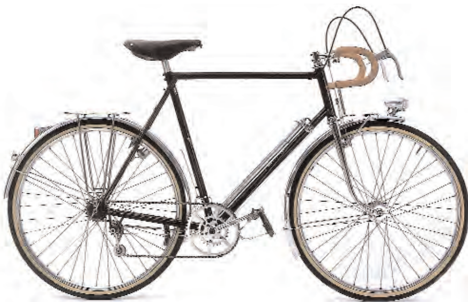
Inspired by the technical trials, this 1947 Alex Singer “light randonneur” bike features a superlight front derailleur, cam-actuated brakes, a tubular aluminum rear rack and many other special parts.
