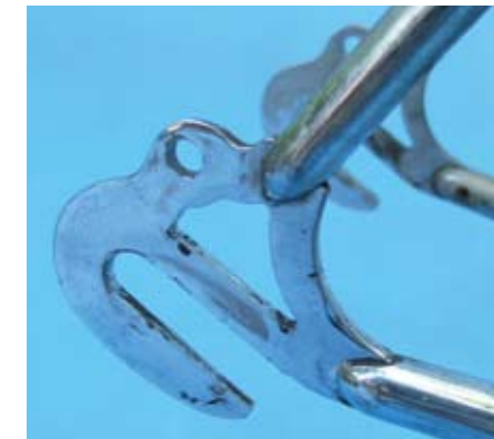
In 1965, very few frames had derailleur hangers on the rear dropouts. The derailleur had its own clamp.
