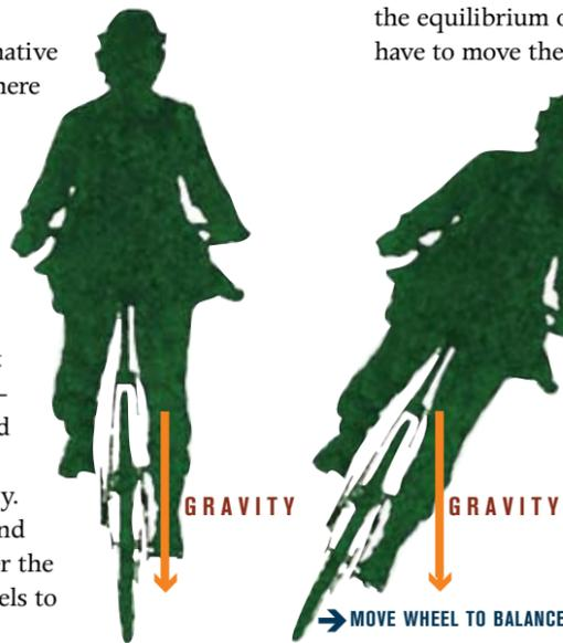
Figure 1: A bicycle is balanced by constantly moving the wheels to keep them under the center of gravity.
